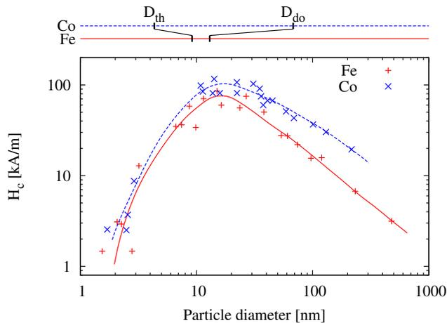
Figure 4: Experimental relation between diameter and coercive field for particles deriving their coercive field principally from crystal anisotropy energy. Measured at a temperature of  $76K$ . Adapted from [6, figure 2], where data was collected from various sources. Theoretical critical diameters as derived here are indicated on top.
